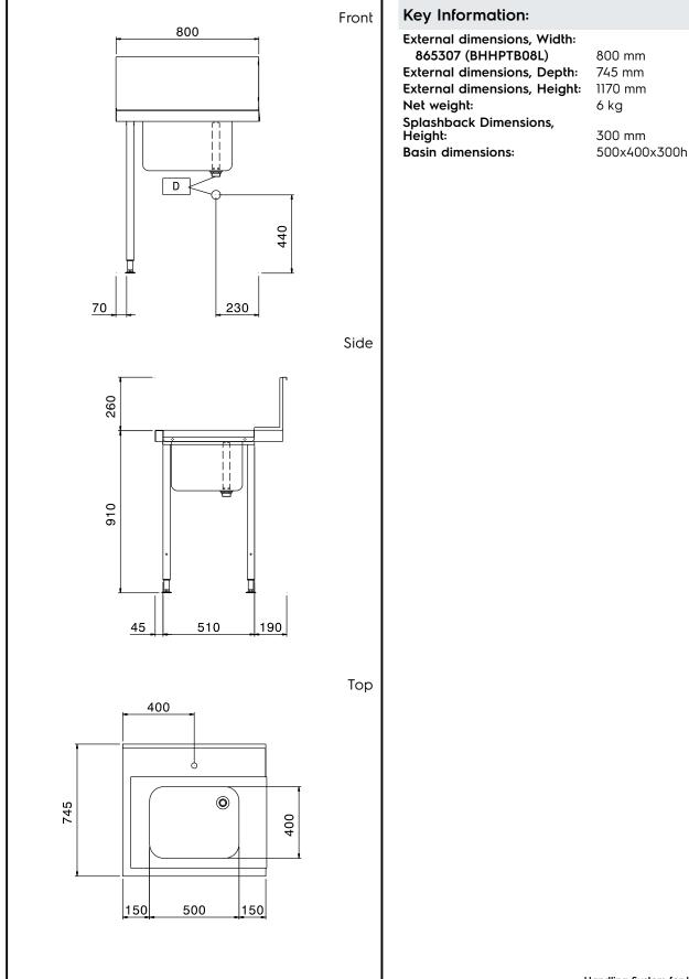
Handling System for Hood type Pre-wash Table with Bowl Left to Right, 800mm
